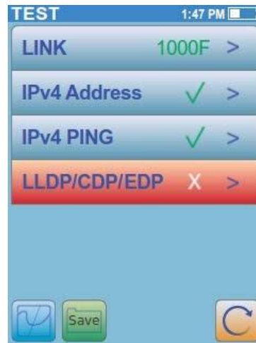
Main Auto Test Screen Failed
