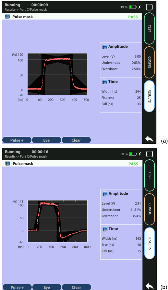
Figure 3.5: xGenius pulse shape analysis panel: (a) E1 pulse mask, (b) T1 pulse mask.
