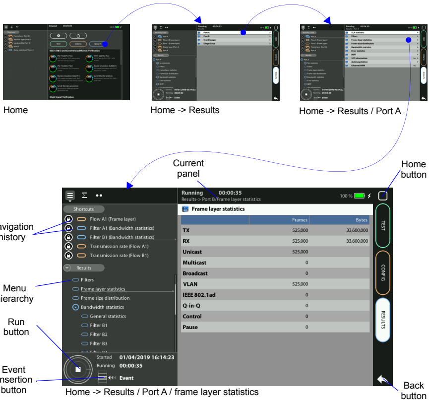
Figure 1.5: Access to a results table from the home panel in three different steps. In this case the test results are represented as a table, including a header (frames, bytes), a results list (TX, RX, ...) and different counters.
