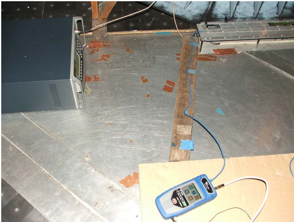
PHOTOGRAPH OF THE TEST SETUP FOR FAST TRANSIENT COMMON MODE TEST (DATA LINES)
