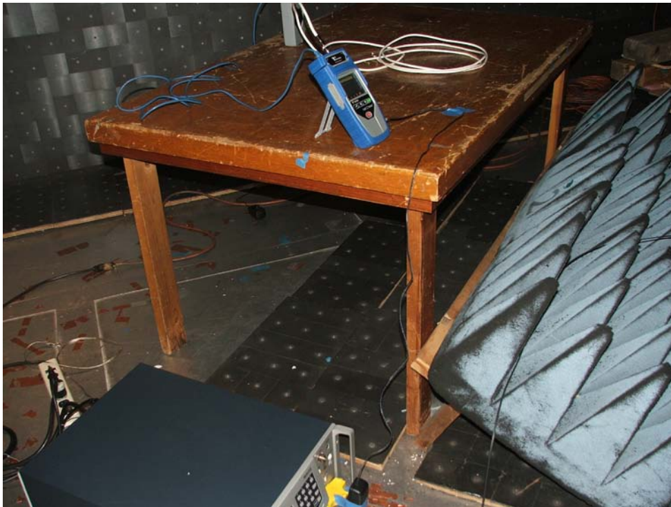
PHOTOGRAPH OF THE TEST SETUP FOR SURGE IMMUNITY TEST (AC INPUT)
