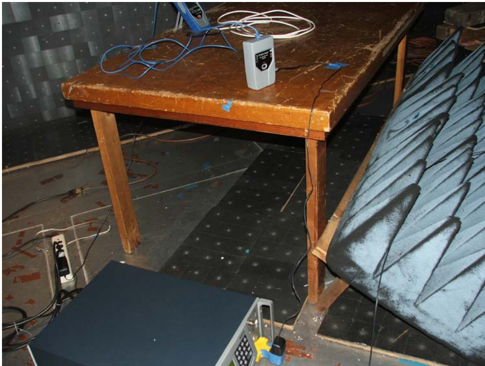
PHOTOGRAPH OF THE TEST SETUP FOR VOLTAGE DIPS & VOLTAGE VARIATIONS AND SHORT INTERRUPTIONS
