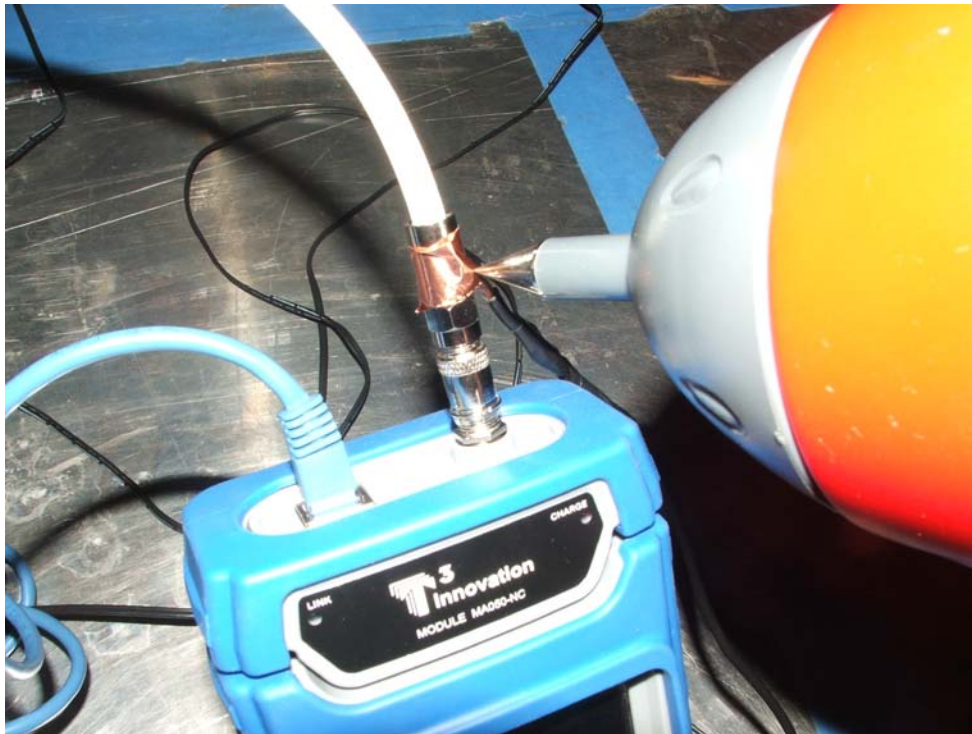
PHOTOGRAPH OF THE TEST SETUP FOR DIRECT ELECTROSTATIC DISCHARGE TEST (CONTACT DISCHARGE)
